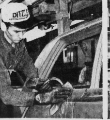
4. Wet Sanding. Following the dip, the car is spray-primed again. After baking, it is meticulously wet sanded by hand to remove all trace of blisters and imperfection from its surface.
