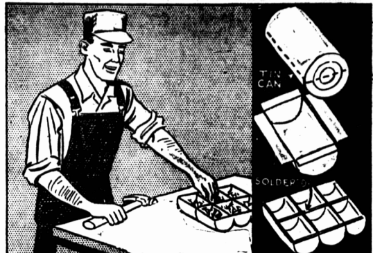
SECTIONAL TRAY... Discarded tin cans of uniform size, preferably the type in which condensed milk is sold, can be cut in the manner indicated in drawing and then crimped and soldered together to make storage trays that will be useful for storing various small parts.
