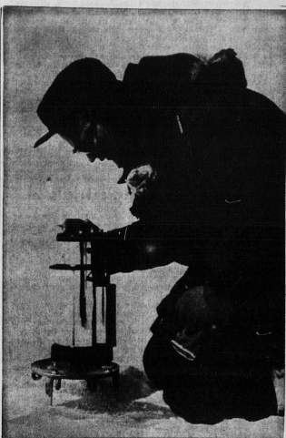
LARRY SOBZEKAK of Ottawa, on loan to the Polar Continental Shelf Project by the Dominion Observatory, takes gravity readings five miles apart on a predetermined section of the Arctic Ocean. Gravity readings, when analyzed, give scientists an indication of the type of rock on the polar shelf and formation of the ocean floor. (CP Photo)
