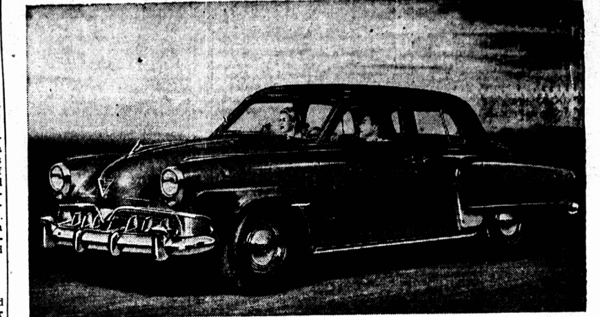
The 1952 Studebaker Land Cruiser. Principal exterior changes of Studebaker's new models include entirely new front-end treatment, new wrap-around grilles and bumpers, re-designed trunk lid handles and tail lights. The latter, by appearing to be integral parts of the fenders rather than "added-on" assemblies, give the effect of extending the sweep of the fenders and the impression of a corresponding increase in body length. Gravel pads on the Land Cruiser, as well as on the State Commander, convertible and "Starliner," are of new design.
