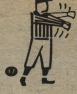
PILING Hands rotated in chopping motion.
