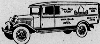
Ford Panel Delivery on 157-inch wheelbase. This is a fully enclosed body for complete protection of bulky loads. Rear doors may be full length, or short with tall gate.
