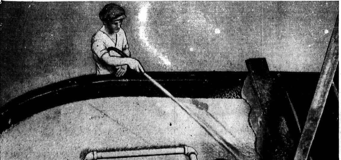
Much of the Sitka spruce goes into pulpwood to make paper or other pulp products. It is cut up, pressed and crushed, made into a wet mash. Above, a worker
