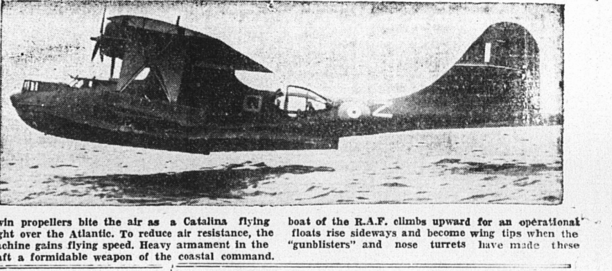
Twin propellers bite the air as a Catalina flying boat rises sideways and become wing tips when the machine gains flying speed. Heavy armament in the craft a formidable weapon of the coastal command.
