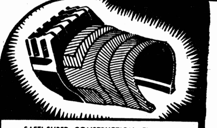
SAFTI-SURED CONSTRUCTION. There are two major parts of a tire - tread and cord body. Safti-Sured Construction means that the tread and cord body are welded together inseparably into a unit of extra strength.
