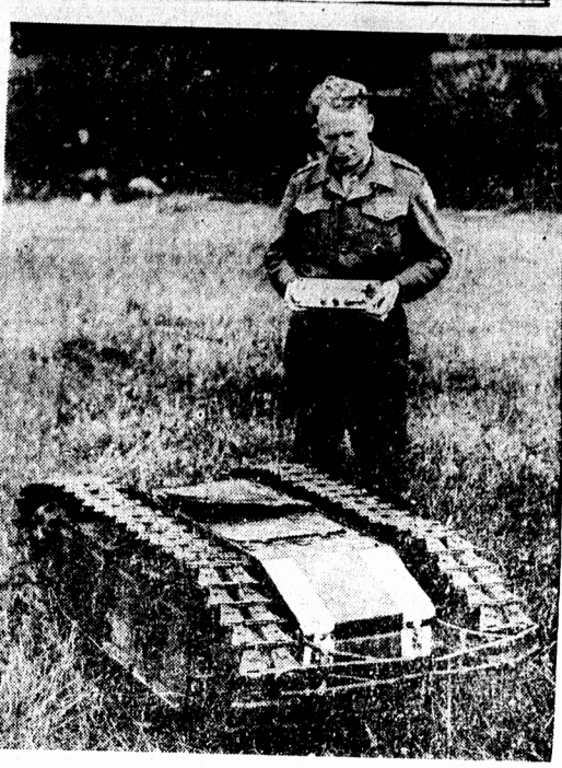
Lieut. Ernest H. Willis, Wolverhampton, Staffordshire, England, with the central box of a captured German Beetle Tank. On the box are buttons to control the movements of the tank and a key to set off the charge when it reaches its objective. (Canadian Army Overseas Photo.)
