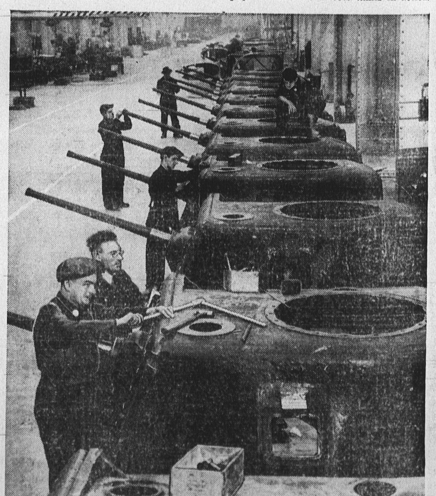
Part of the production line in the Ram tank factory, second largest arsenal for tank production in the world. Heavily armed with machine guns and cannon, the Ram is powered with a Wright Whirlwind engine, a versatile war machine.
