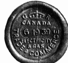
This Government Seal is your guarantee that the meter has been officially approved, inspected and found accurate. The seal also prevents tampering with or manipulation of the meter's mechanism.
