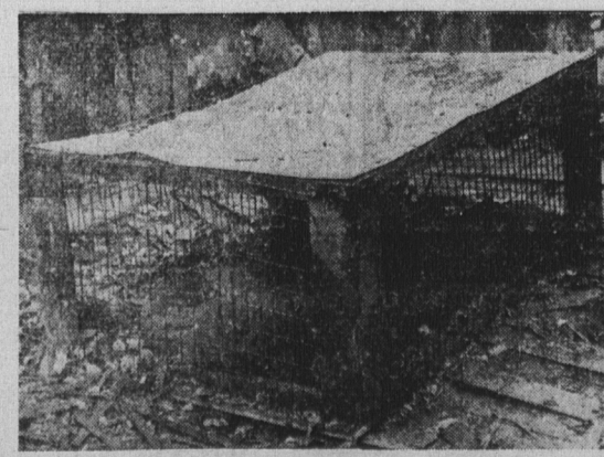
Safe survival for the new low cost air raid shelter, with a flap top like a table and grating-enclosed sides, was the result of the test. Authorities announced the shelters could be given without charge to low-income bracket families. Others may purchase them.
