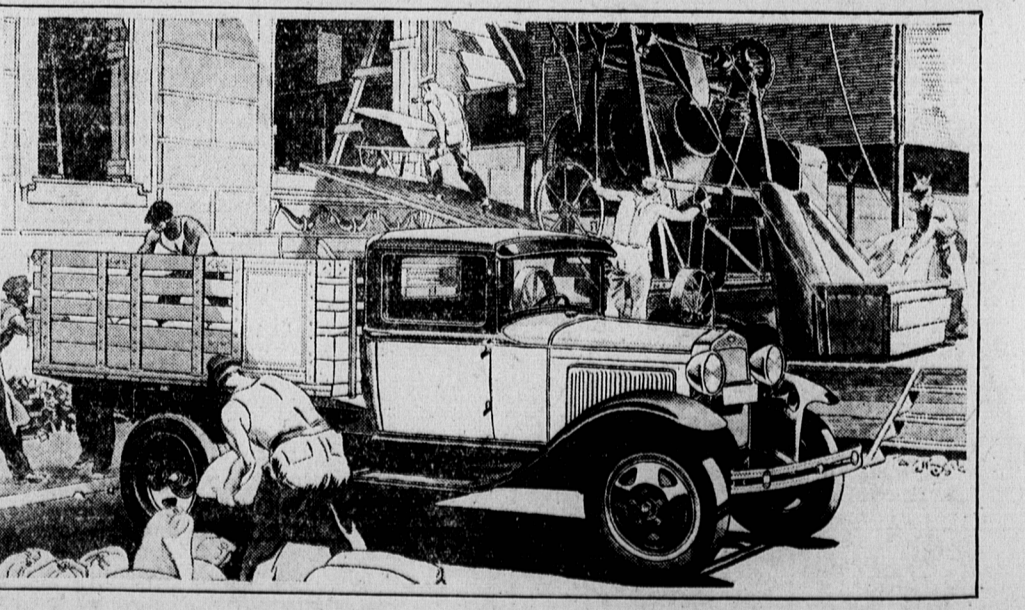
Showing the stake body, and one of its many uses. This type may be installed on the 131 1/2-inch or 157-inch chassis
